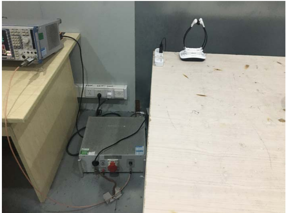
Conducted Emission Test Setup
