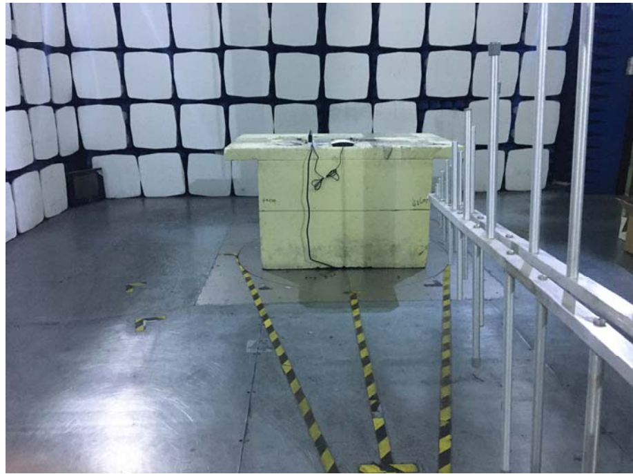
Radiation Emission Test Setup (30MHz to 1GHz)
