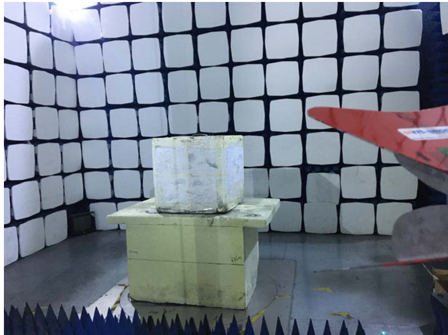
Radiation Emission Test Setup (1GHz to 18GHz)
