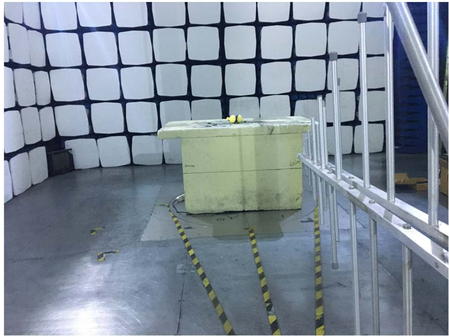
Radiation Emission Test Setup (30MHz to 1GHz)
