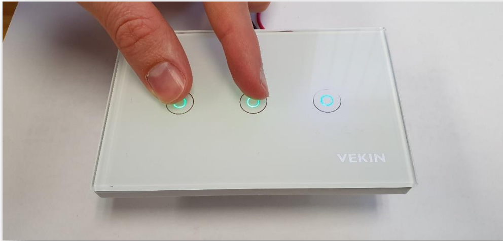
Figure 9: Hold down the left and middle button (>15s) to erase the previously paired iOS device
