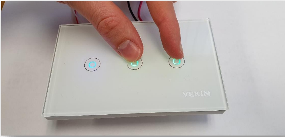
Figure 12: Hold down the middle and right button (>15s) to erase the previously paired android device
