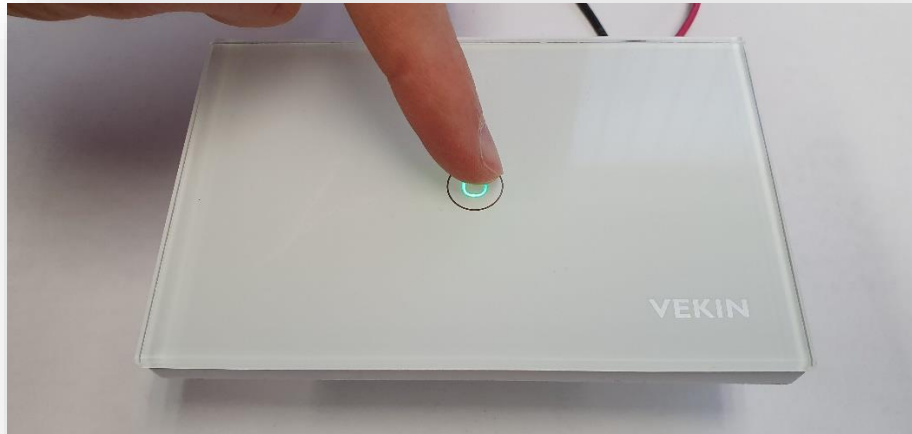
Figure 2: Hold down the button (>30s) to enter network configuration mode
