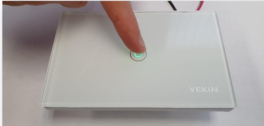
Figure 7: Hold down the button (>15s, release before 30s) to erase the previously paired iOS device
