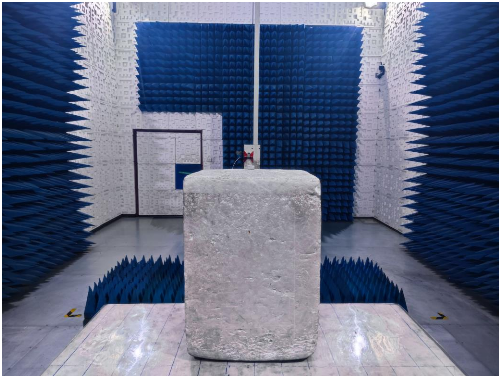
RADIATED EMISSION TEST SETUP ABOVE 1GHz
