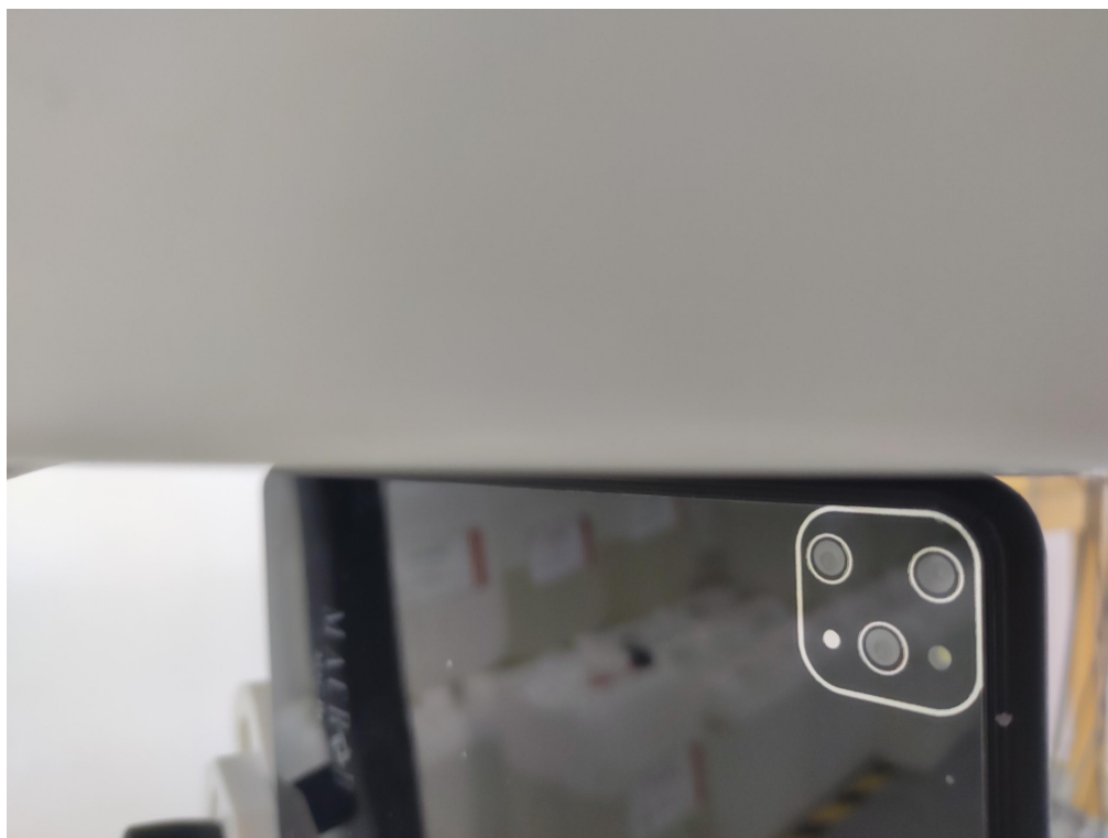
0mm body-worn Right Side Setup Photo (hotspot)
