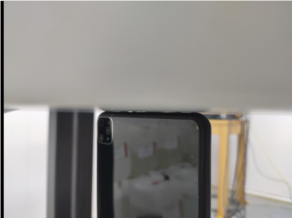
0mm body-worn Top Side Setup Photo (hotspot)
