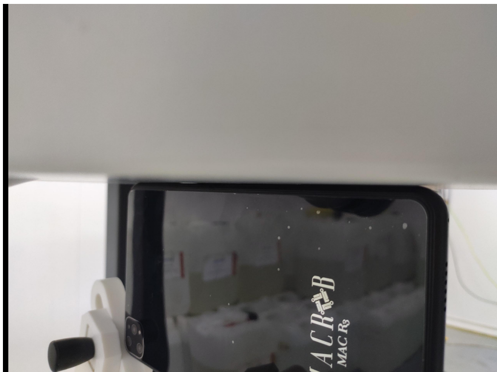
0mm body-worn Left Side Setup Photo (hotspot)
