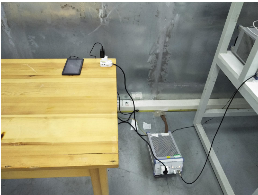
AC Conducted Emission of charge from power
