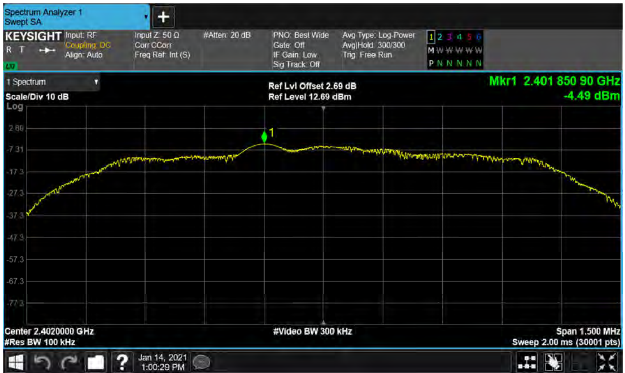
Tx. Spurious NVHT 2-DH1 2402MHz Ant1 Ref
