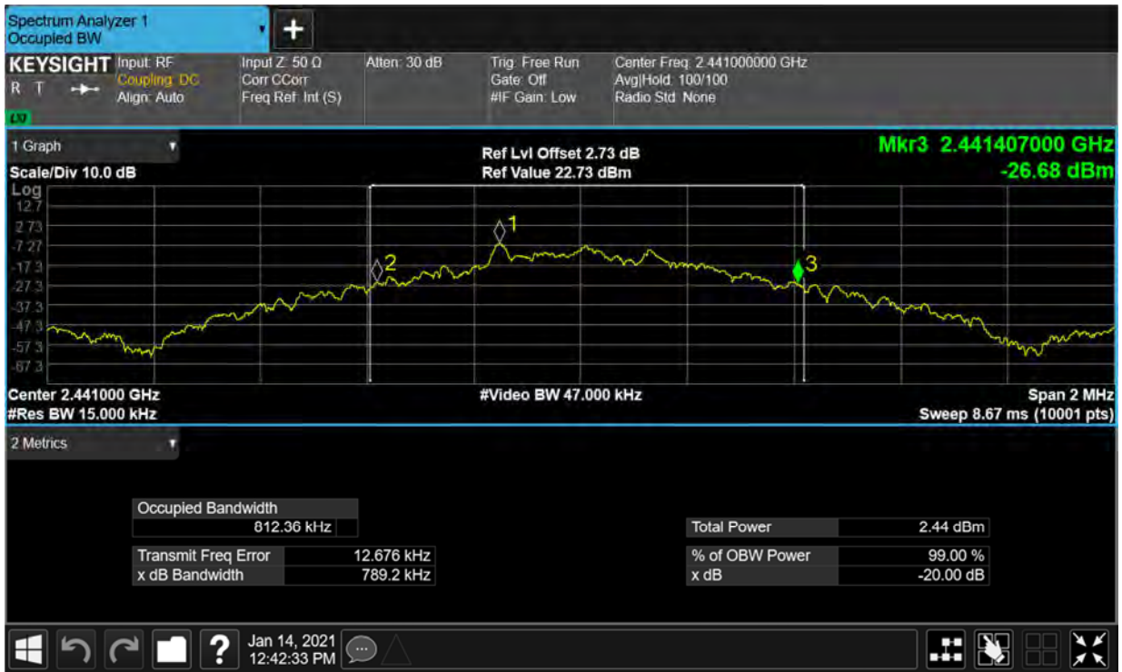
-20dB Bandwidth NVHT 1-DH1 2441MHz Ant1
