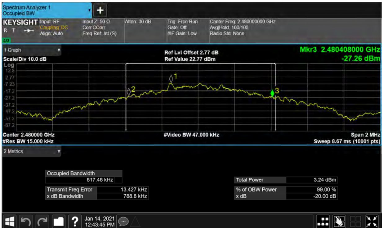
-20dB Bandwidth NVHT 1-DH1 2480MHz Ant1
