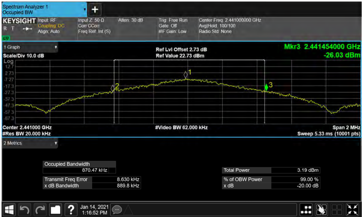
-20dB Bandwidth NVHT 3-DH1 2441MHz Ant1
