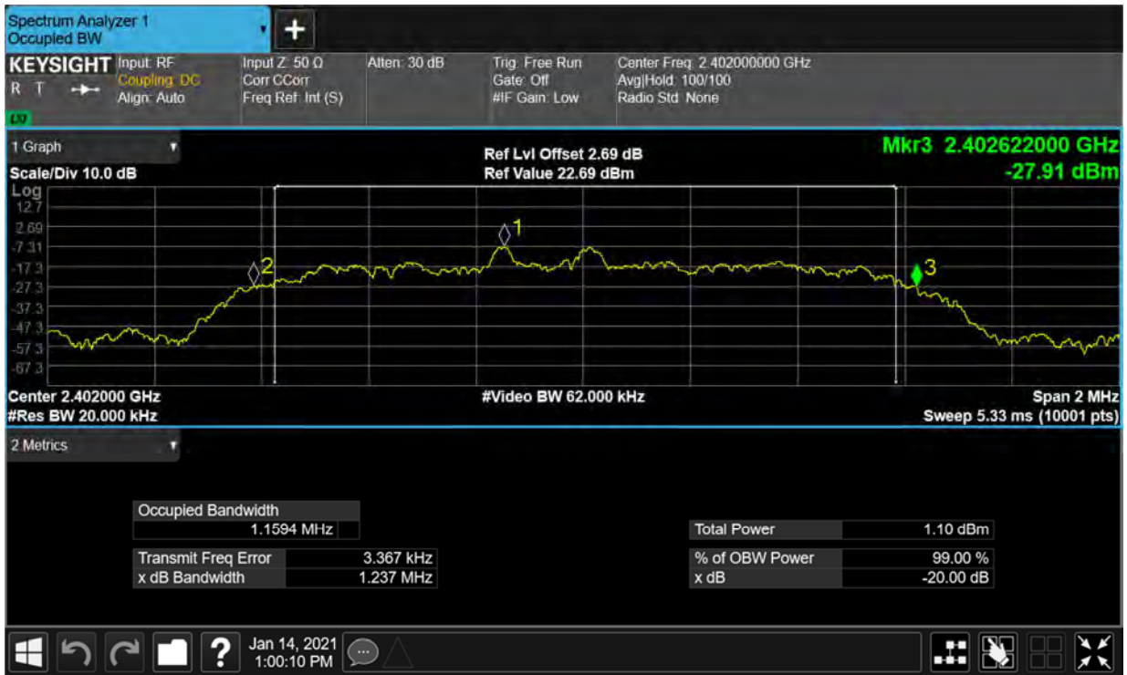
-20dB Bandwidth NVHT 2-DH1 2402MHz Ant1
