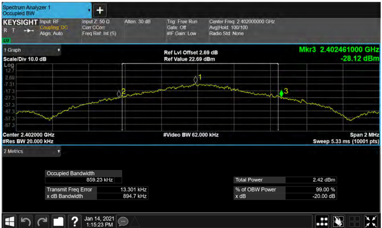
-20dB Bandwidth NVHT 3-DH1 2402MHz Ant1
