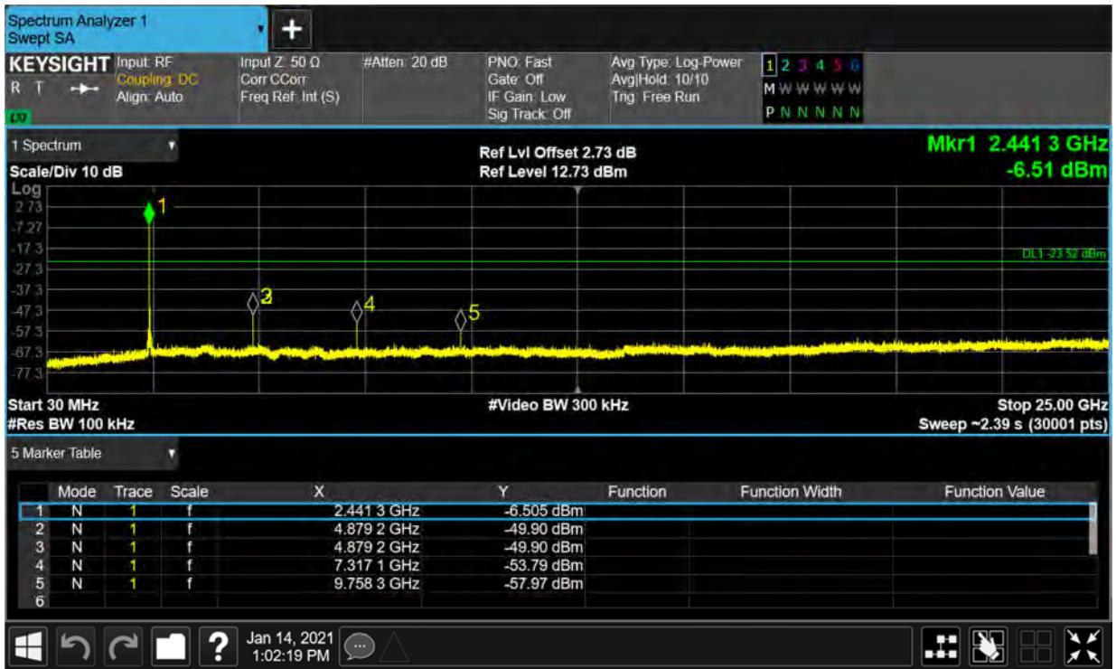
Tx. Spurious NVHT 2-DH1 2441MHz Ant1 Emission
