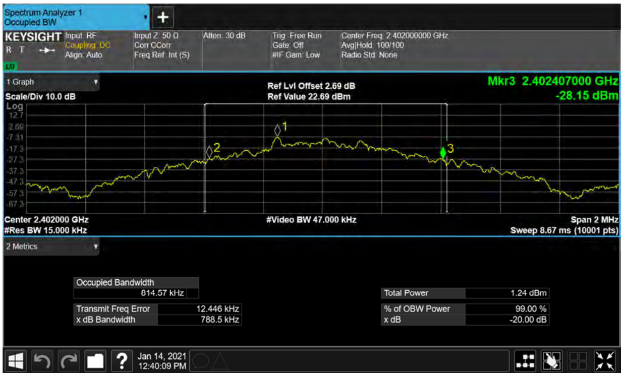
-20dB Bandwidth NVHT 1-DH1 2402MHz Ant1
