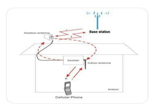
If isolation can't be achieved by the limited distance, the roof of the building or any other barriers can be used in between to increase isolation.
