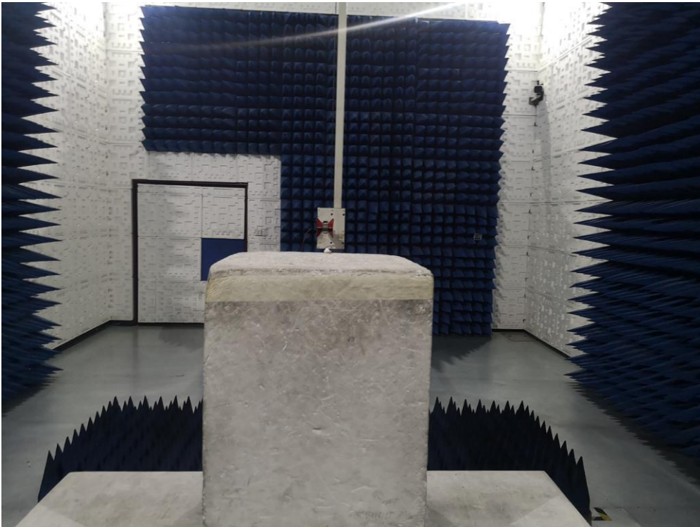
RADIATED EMISSION TEST SETUP ABOVE 1GHz
