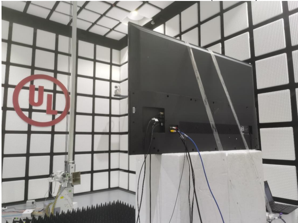
RADIATED RF MEASUREMENT SETUP (Above 1G )
