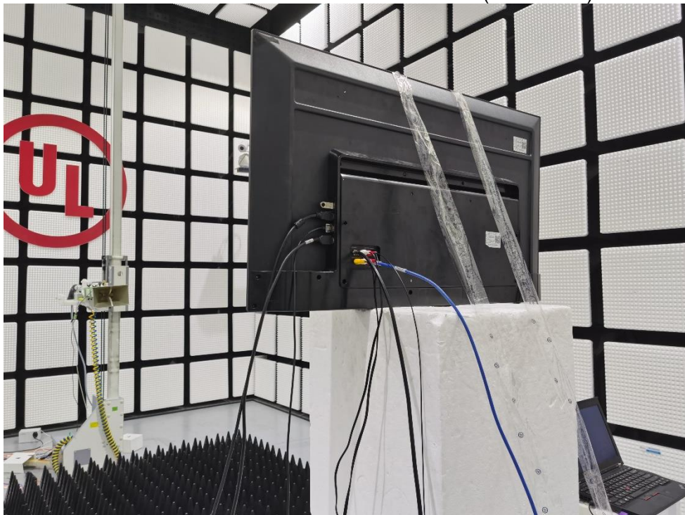
RADIATED RF MEASUREMENT SETUP (Above 1G )
