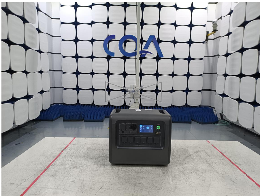
Below 30MHz Test Setup
