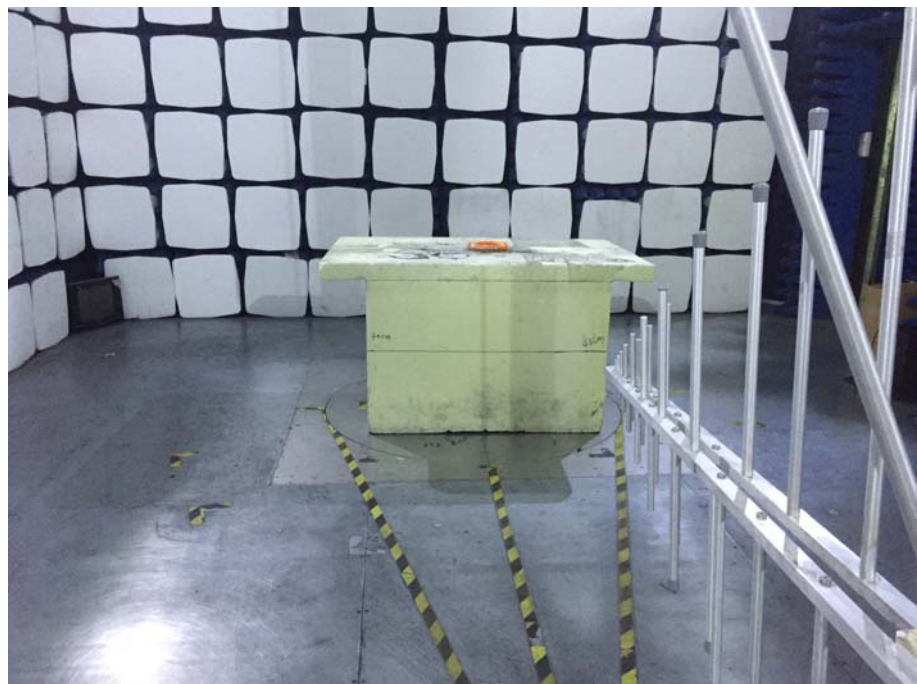
Radiation Emission Test Setup (30MHz to 1GHz)
