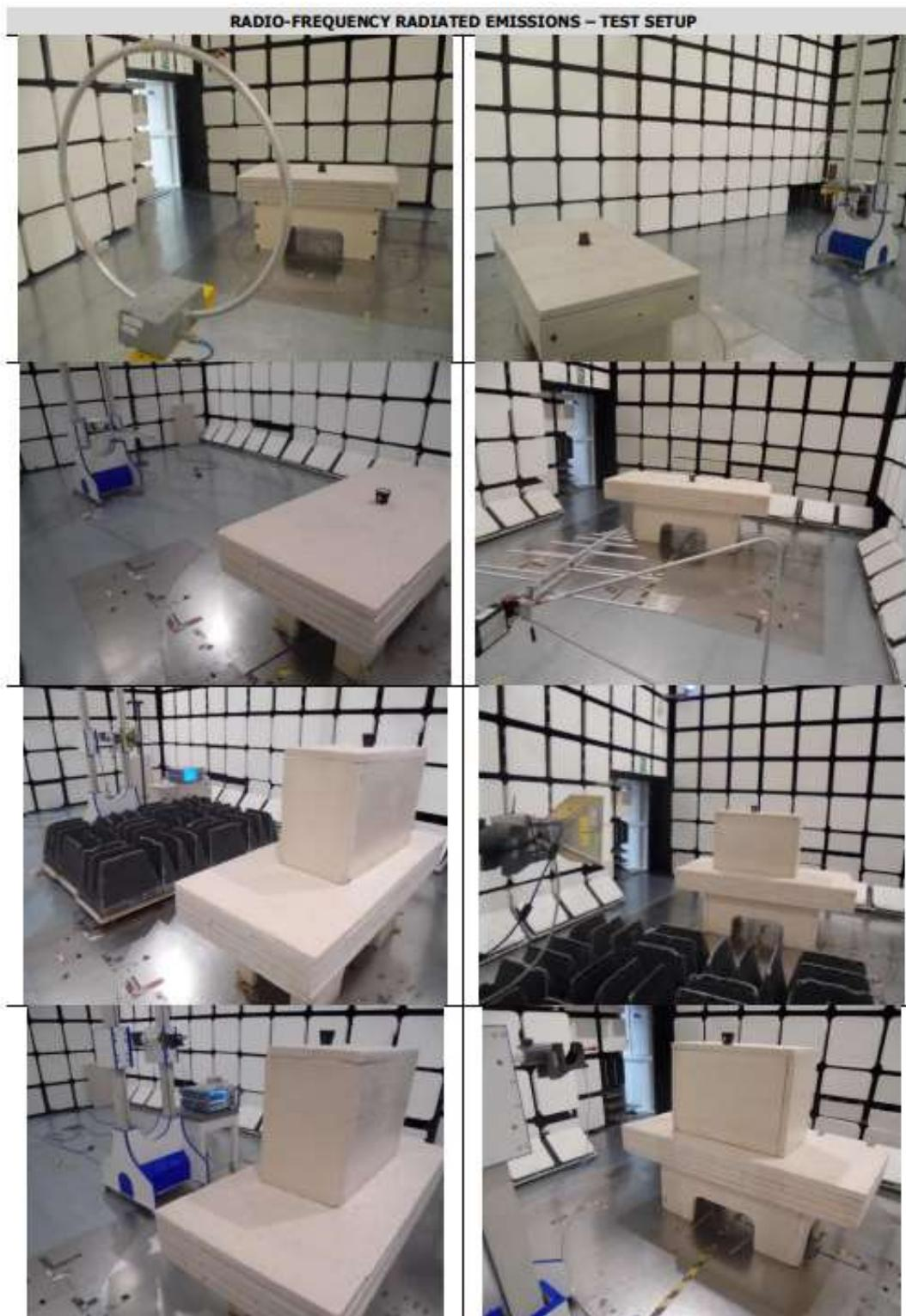
Part 15B Radiated Test Set-up
