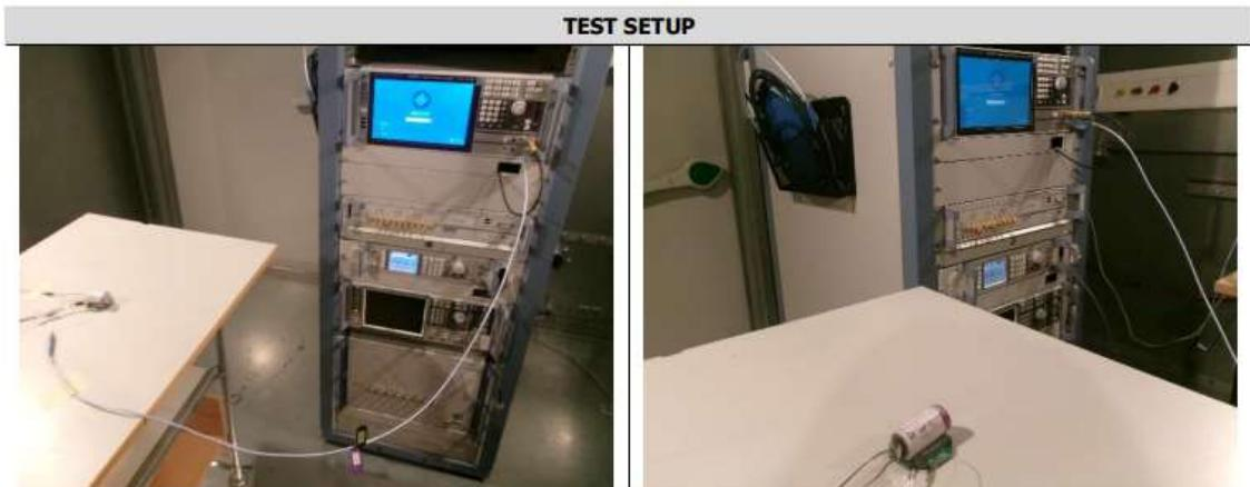
Part 15C Radiated Test Set-up
