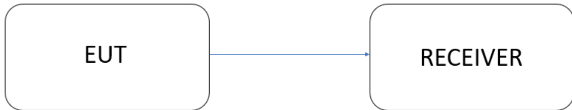
Fig. 1: Occupied Channel Bandwidth setup of tabletop equipment
