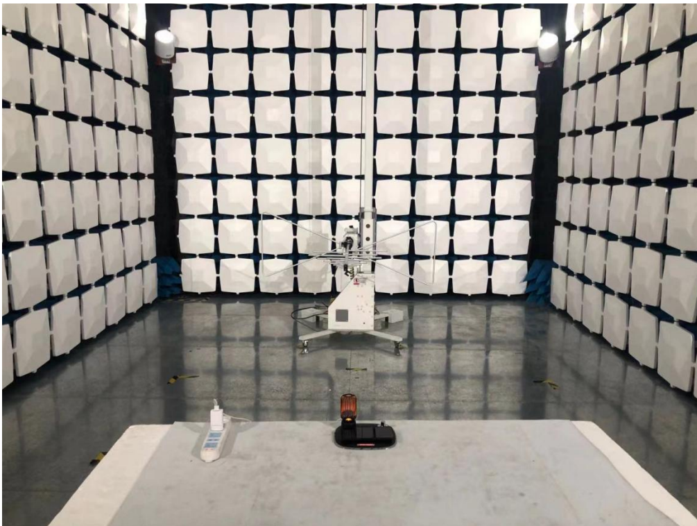
Blow 1GHz for radiated emission test setup
