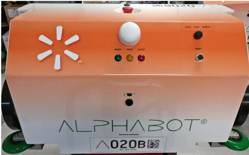
Status Lights, WiFi Antennae, and Service Switch
