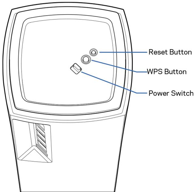
**Reset button**—Press and hold until the light on top of the node turns red, fades and flashes bright red again to reset the node to its factory defaults.
