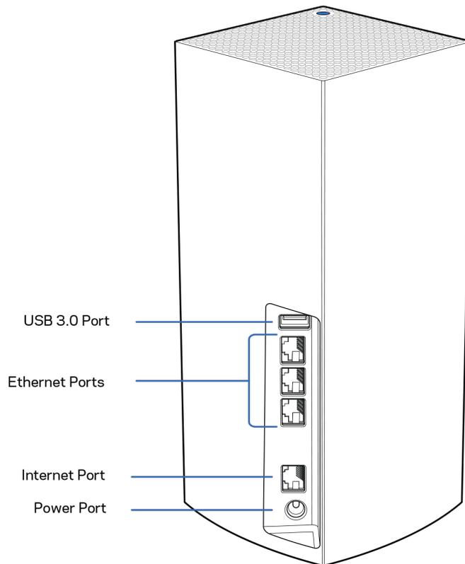
**USB 3.0 port**— Connect and share USB drives on your network. For local file sharing only (no FTP, media server or virtualUSB support). Also, not intended for sharing peripherals such as printers, scanners or cameras.
