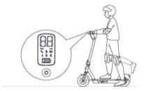
Release the speed controller to slow down; squeeze the braking handle to brake.
