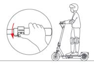
Check battery frequently, charge the battery when power is low. Stand on the pedal with one foot and push off with another foot to start gliding.
