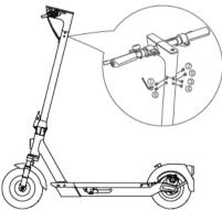
Install the handlebar on the front tube in the correct direction.
