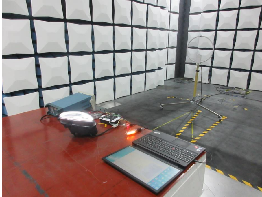
RADIATED RF MEASUREMENT SETUP (9kHz ~ 30 MHz)
