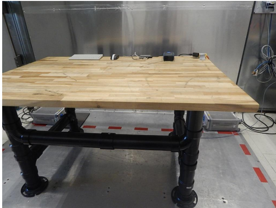
Figure 7.1-5: Conducted emissions – from AC mains power ports setup photo
