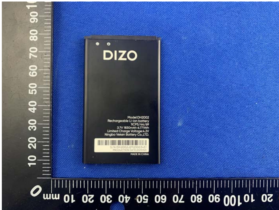
Battery Photo (FRONT)
