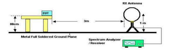
2. Radiated Emission Test Set-Up, Frequency Below 1000 MHz
