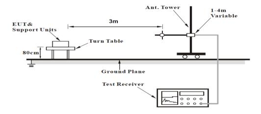
3. Radiated Emission Test Set-Up, Frequency Above 1000 MHz.
