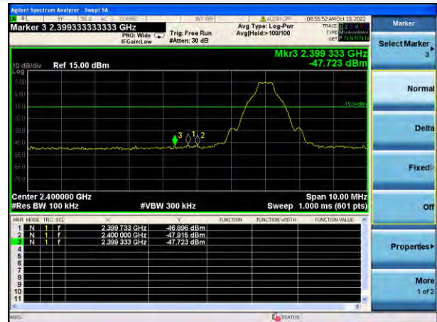
GFSK LOW CHANNEL, BAND EDGE
