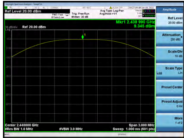
GFSK (BLE 1Mbps) MIDDLE CHANNEL
