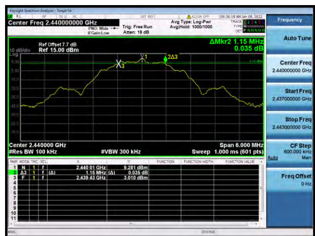
GFSK (BLE 2Mbps) MIDDLE CHANNEL
