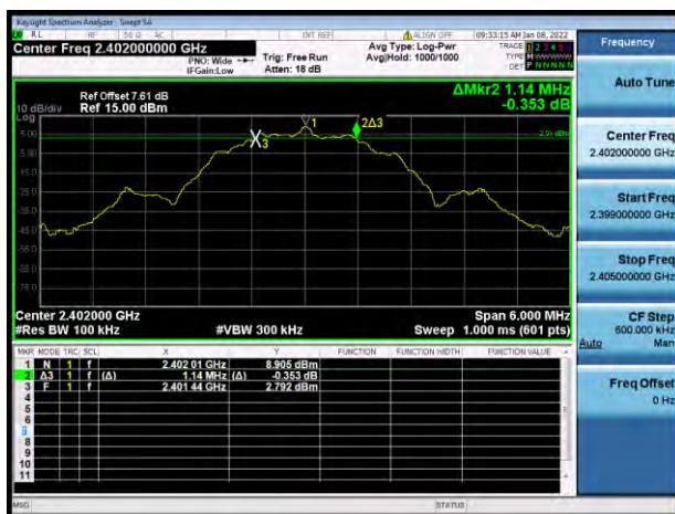
GFSK (BLE 2Mbps) LOW CHANNEL
