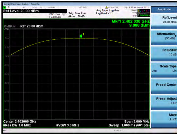
GFSK (BLE 1Mbps) LOW CHANNEL
