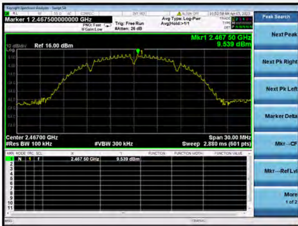
802.11b CHANNEL 12, CARRIER LEVEL
