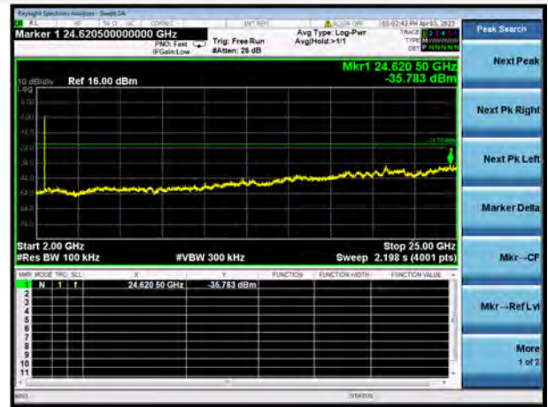
802.11ax-20 MHz(SU) CHANNEL 13, SPURIOUS 2 GHz ~ 25 GHz
