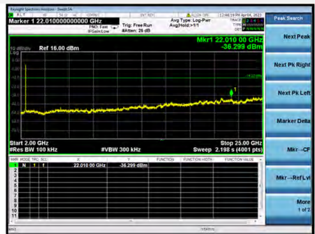
802.11ax-20 MHz(SU) CHANNEL 11, SPURIOUS 2 GHz ~ 25 GHz
