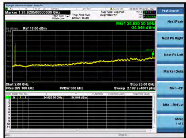
802.11ax-40 MHz(SU) CHANNEL 10, SPURIOUS 2 GHz ~ 25 GHz
