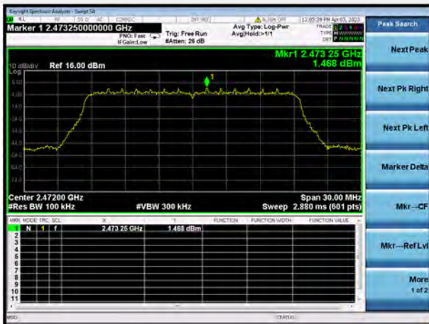
802.11ax-20 MHz(SU) CHANNEL 13, CARRIER LEVEL
