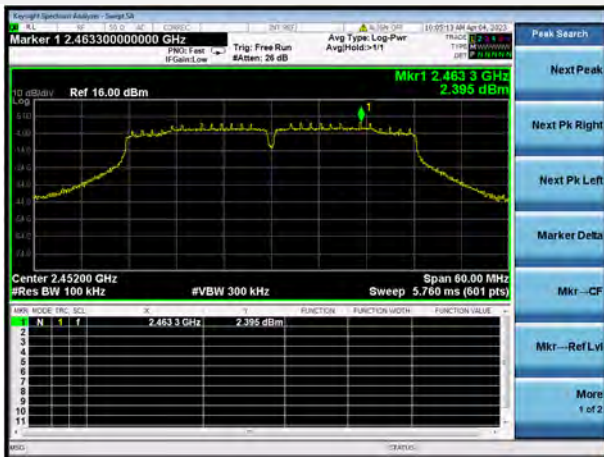
802.11n-40 MHz CHANNEL 9, CARRIER LEVEL
