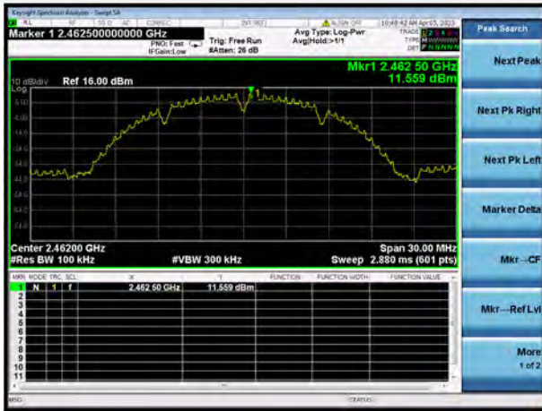
802.11b CHANNEL 11, CARRIER LEVEL
