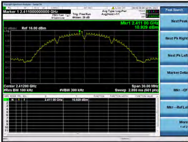
802.11b CHANNEL 1, CARRIER LEVEL
