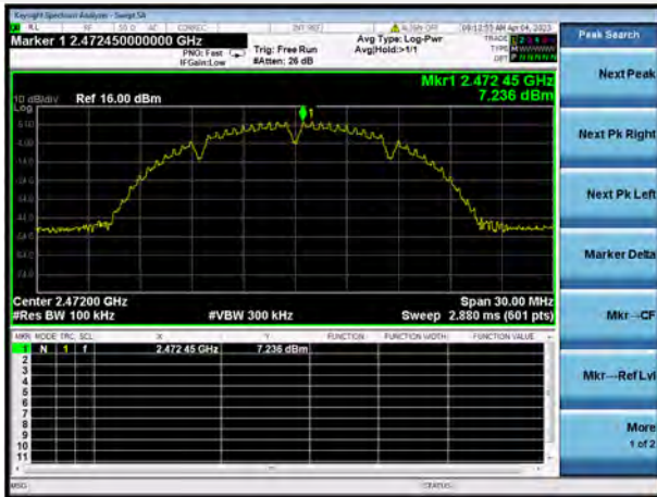
802.11b CHANNEL 13, CARRIER LEVEL
