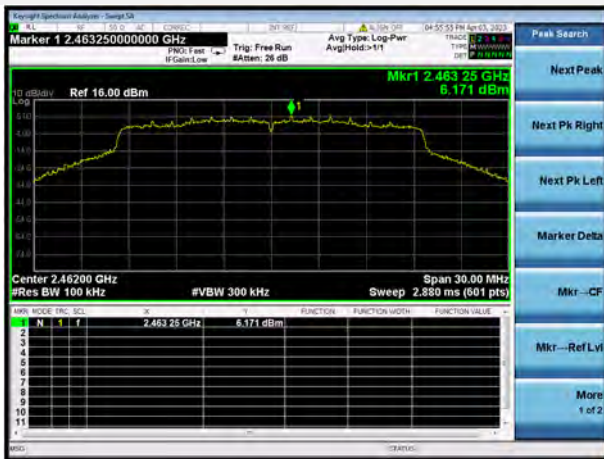
802.11ax-20 MHz(SU) CHANNEL 11 CARRIER LEVEL
