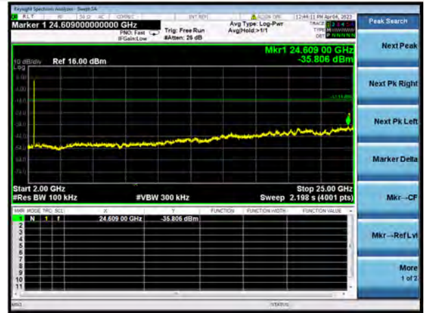
802.11ax-20 MHz(SU) CHANNEL 6, SPURIOUS 2 GHz ~ 25 GHz
