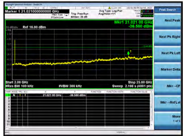
802.11ax-40 MHz(SU) CHANNEL 9, SPURIOUS 2 GHz ~ 25 GHz
