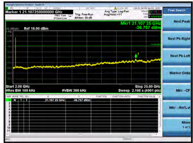
802.11ax-20 MHz(SU) CHANNEL 6, SPURIOUS 2 GHz ~ 25 GHz
