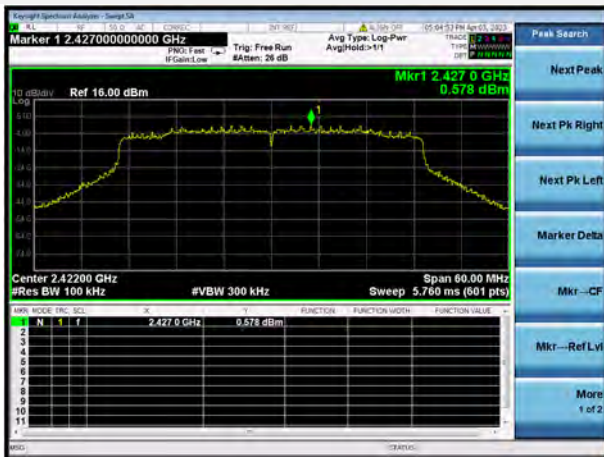
802.11ax-40 MHz(SU) CHANNEL 3, CARRIER LEVEL
