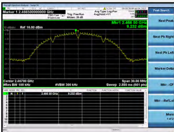
802.11b CHANNEL 12, CARRIER LEVEL
