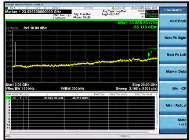
802.11ax-20 MHz(SU) CHANNEL 13, SPURIOUS 2 GHz ~ 25 GHz
