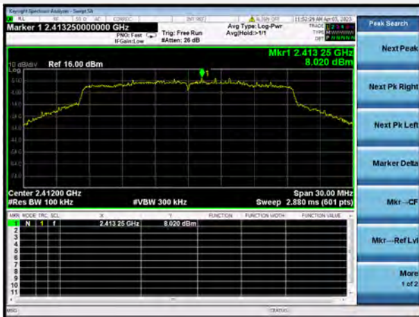
802.11ax-20 MHz(SU) CHANNEL 1, CARRIER LEVEL
