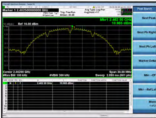
802.11b CHANNEL 11, CARRIER LEVEL
