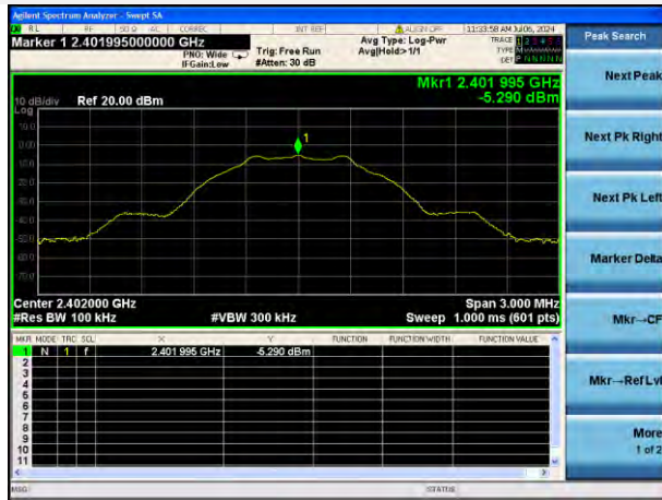
GFSK (BLE 1Mbps) LOW CHANNEL, CARRIER LEVEL
