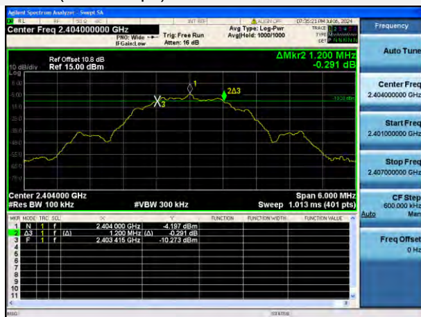
GFSK (BLE 2Mbps) LOW CHANNEL
