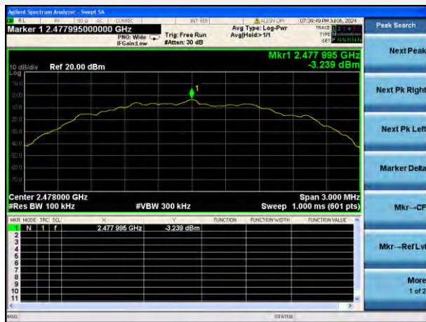
GFSK (BLE 2Mbps) HIGH CHANNEL, CARRIER LEVEL
