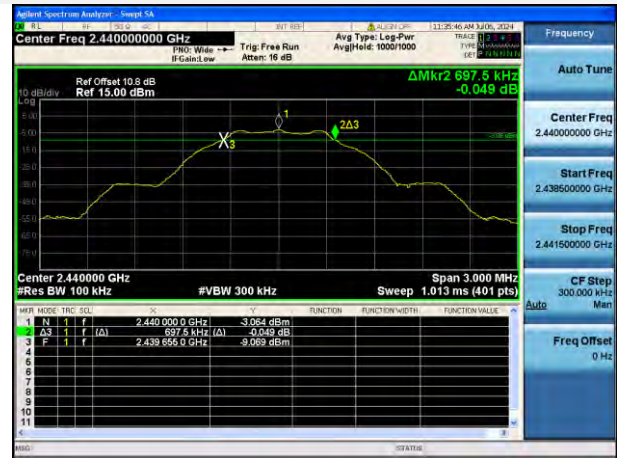
GFSK (BLE 1Mbps) MIDDLE CHANNEL
