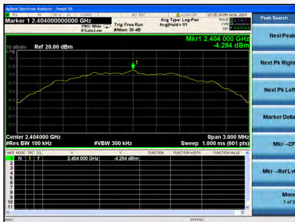
GFSK (BLE 2Mbps) LOW CHANNEL, CARRIER LEVEL
