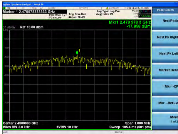
GFSK (BLE 1Mbps) HIGH CHANNEL
