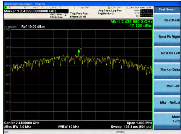
GFSK (BLE 1Mbps) MIDDLE CHANNEL
