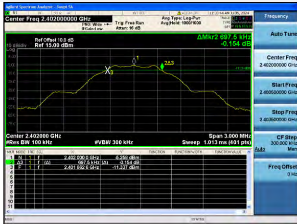
GFSK (BLE 1Mbps) LOW CHANNEL
