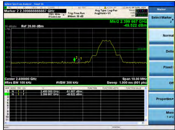
GFSK (BLE 1Mbps) HIGH CHANNEL, BAND EDGE
