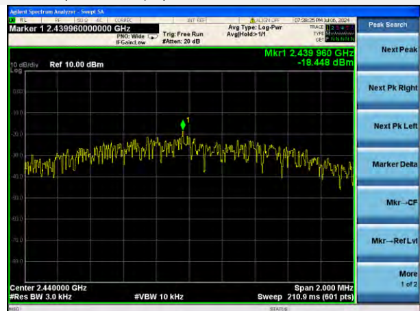
GFSK (BLE 2Mbps) MIDDLE CHANNEL
