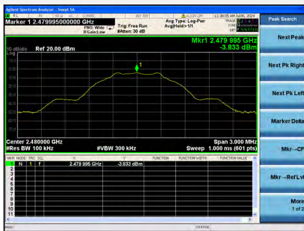
GFSK (BLE 1Mbps) HIGH CHANNEL, CARRIER LEVEL
