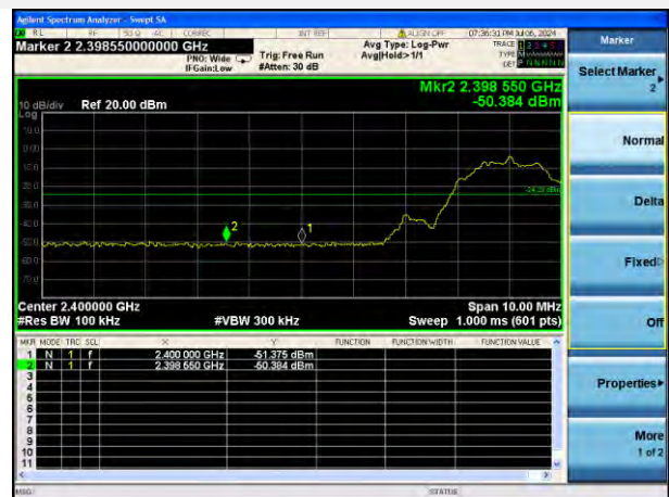
GFSK (BLE 2Mbps) LOW CHANNEL, BAND EDGE
