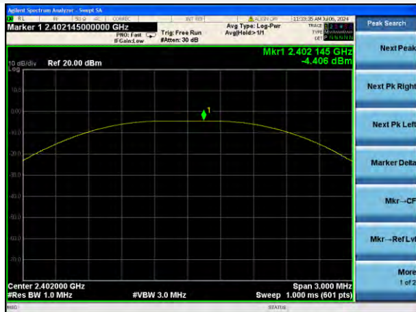
GFSK (BLE 1Mbps) LOW CHANNEL
