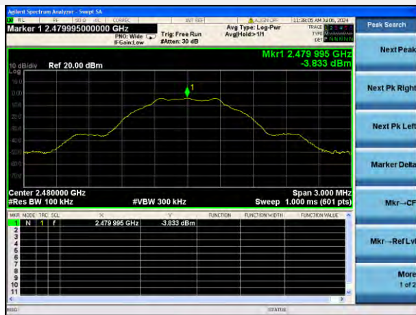
GFSK (BLE 1Mbps) HIGH CHANNEL, CARRIER LEVEL
