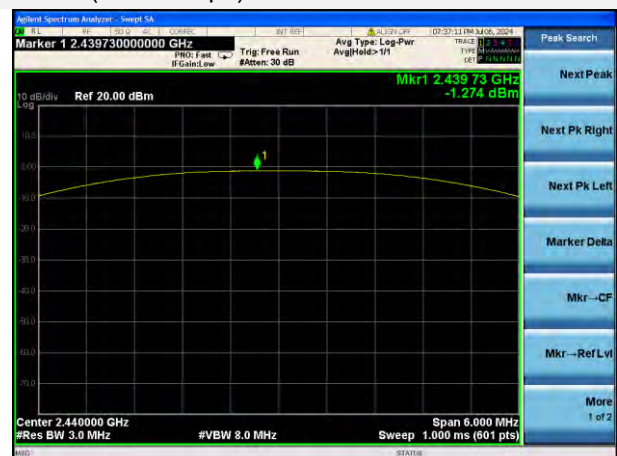
GFSK (BLE 2Mbps) MIDDLE CHANNEL
