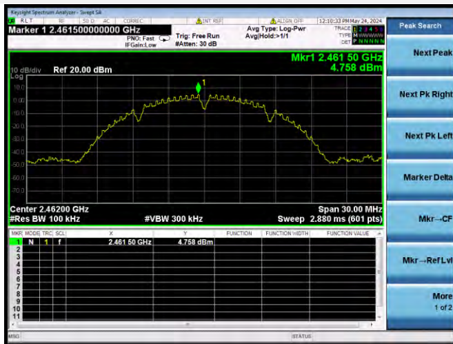
802.11b HIGH CHANNEL, CARRIER LEVEL
