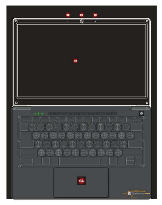
Attention:Do NOT open the display panel beyond 135 degrees When closing the display panel, and Do NOT leave pens or any other objects between the display panel and the keyboard.Otherwise, the display panel may be damaged.
