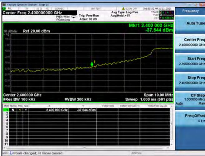
802.11g LOW CHANNEL, Carrier level
