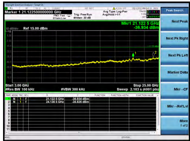
GFSK LOW CHANNEL, SPURIOUS 3 GHz ~ 25 GHz
