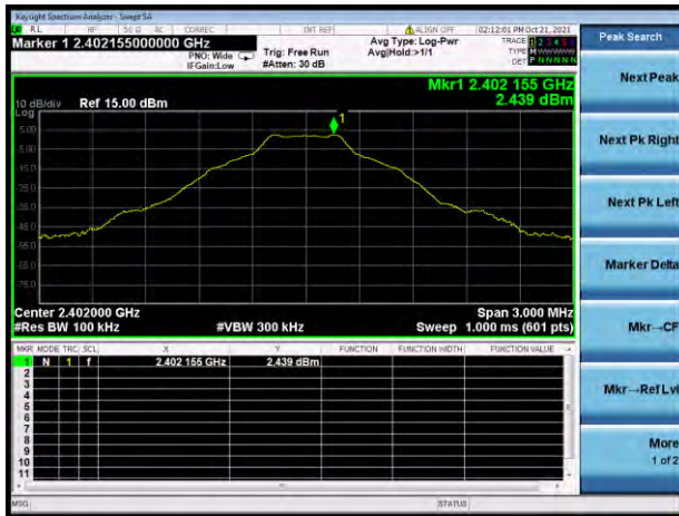
GFSK LOW CHANNEL, CARRIER LEVEL
