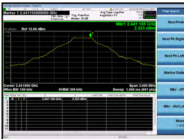
GFSK MIDDLE CHANNEL, CARRIER LEVEL
