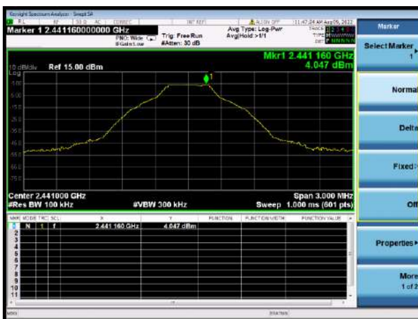
GFSK MIDDLE CHANNEL, CARRIER LEVEL
