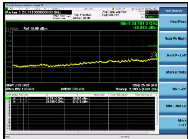
GFSK LOW CHANNEL, SPURIOUS 3 GHz ~ 25 GHz
