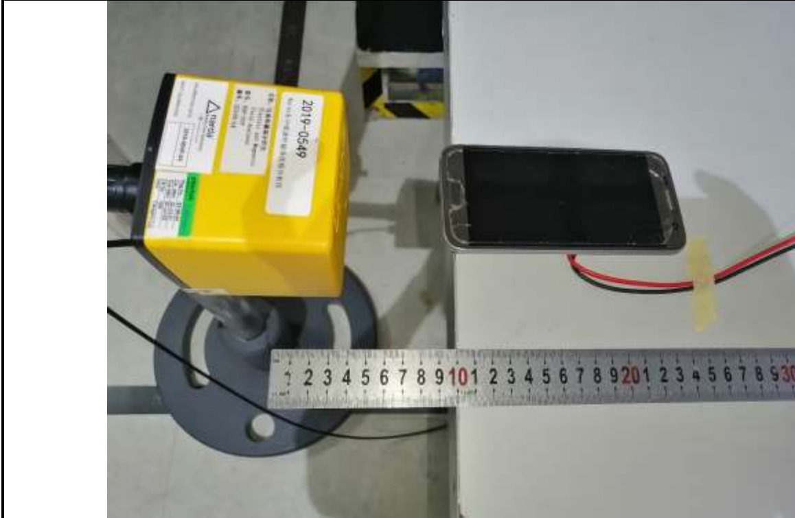
E-Field Strength and H-Field Strength Position B (10cm)
