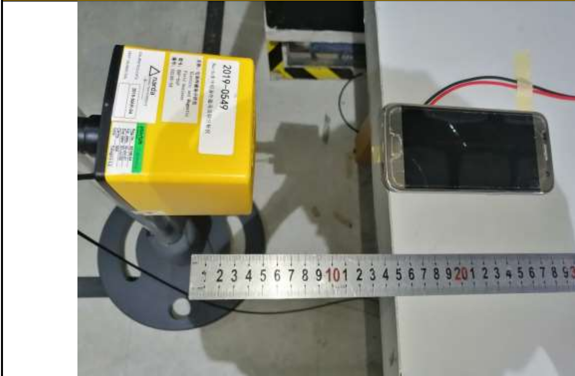
E-Field Strength and H-Field Strength Position A (Distance 15cm)
