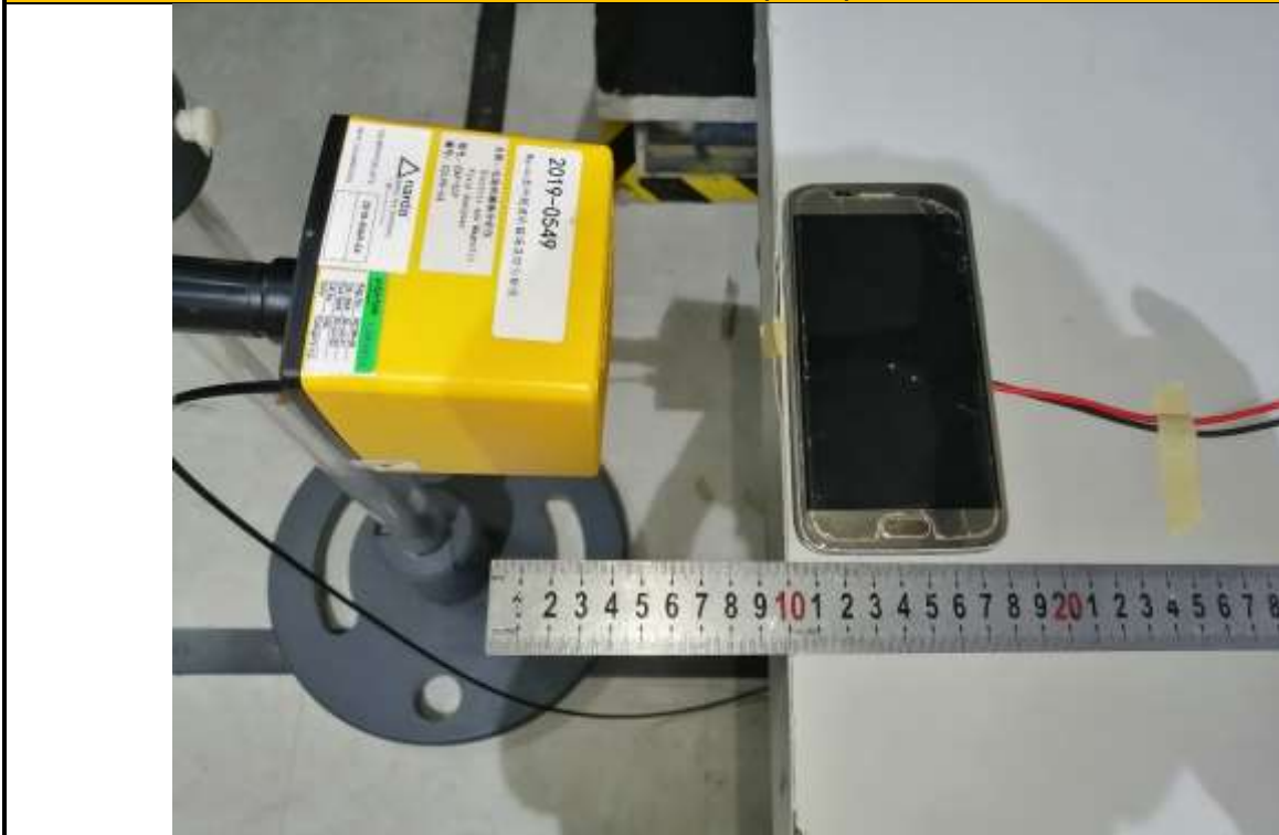
E-Field Strength and H-Field Strength Position C (10cm)
