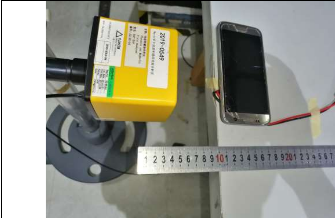
E-Field Strength and H-Field Strength Position D (10cm)
