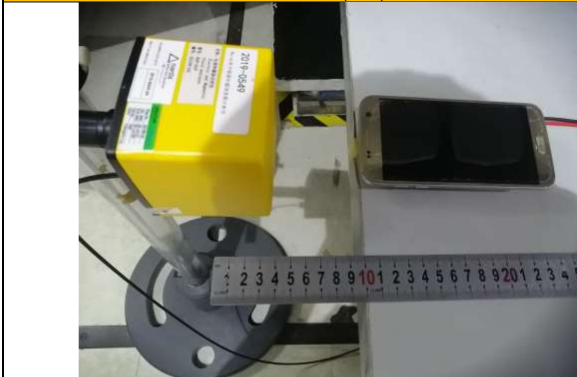
E-Field Strength and H-Field Strength Position A (10cm)
