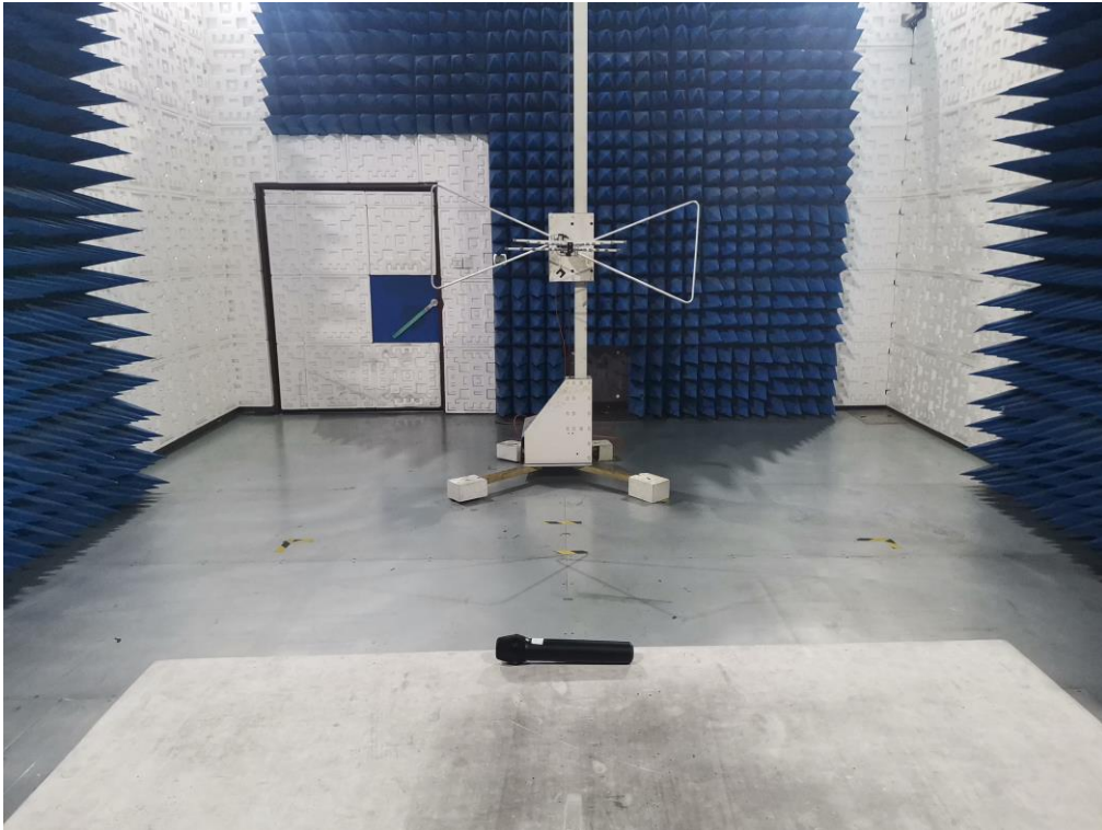
RADIATED EMISSION TEST SETUP ABOVE 1GHZ
