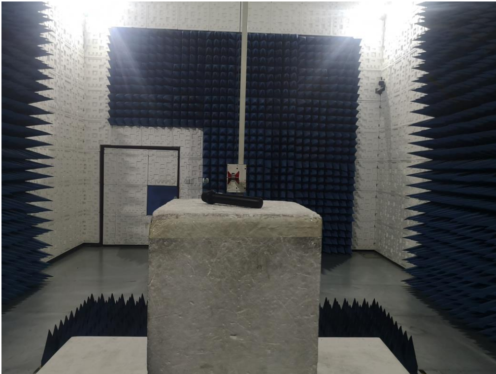
RADIATED EMISSION TEST SETUP ABOVE 1GHZ
