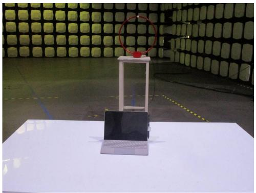
Radiated Emissions (30MHz-1GHz) Test Setup
