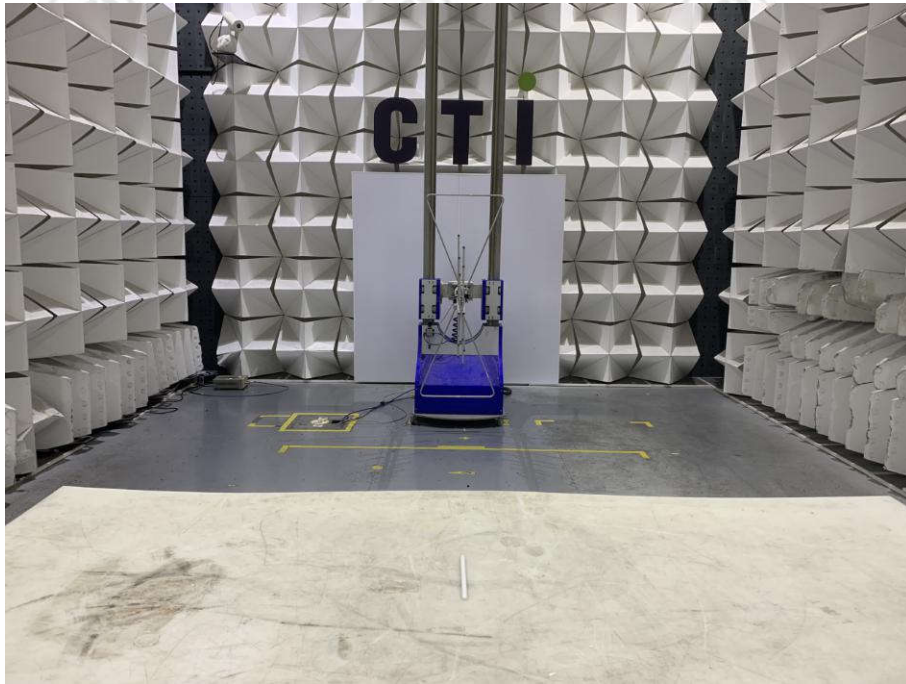
Radiated spurious emission Test Setup-1(Below 1GHz)
