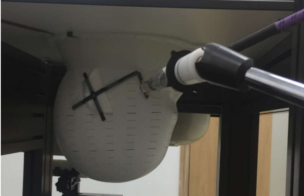
5GHz Dipole Placed at Location C in 90° Orientation (25mm Spacer)
