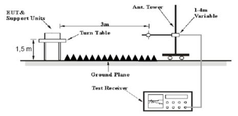
The radiated emission below 1GHz tests were performed in the 3 meters chamber A, above 1GHz tests were performed in the 3 meters chamber A, using the setup accordance with the ANSI C63.10-2013. The specification used was the FCC 15.209, and FCC 15.247 limits.
