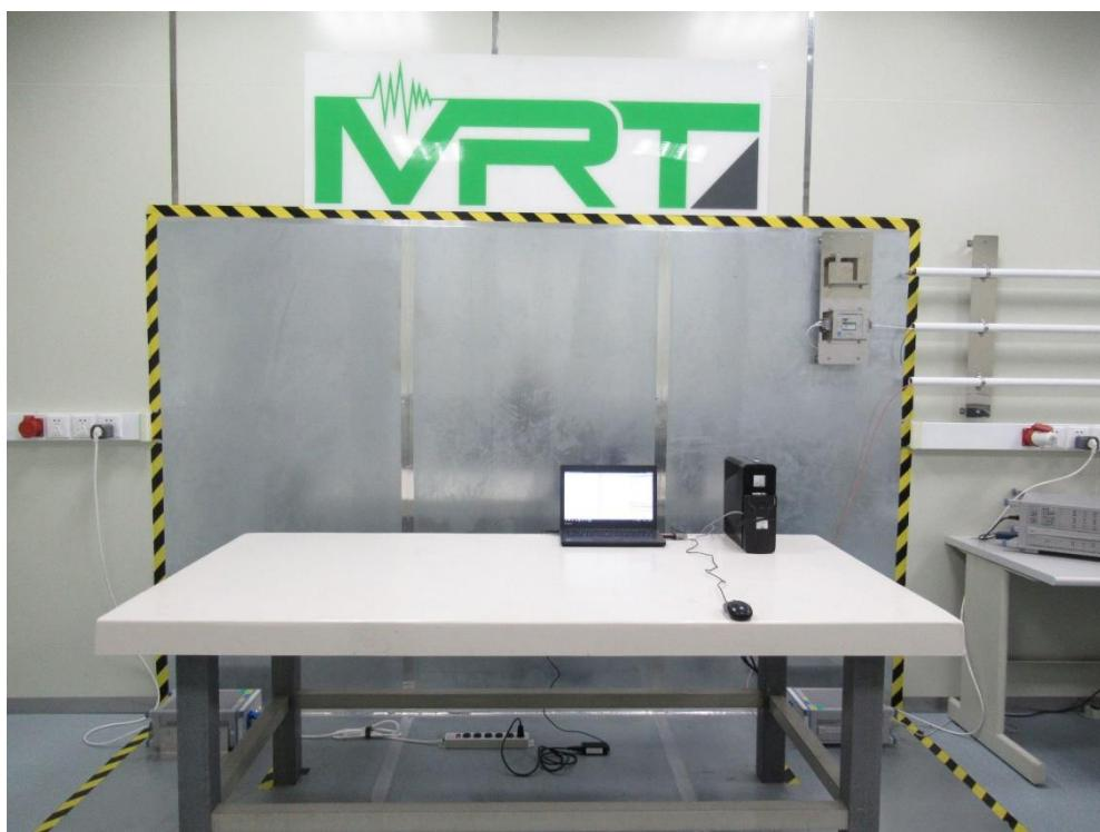
**Test Mode: Mode 2****Description: Back View of Conducted Emission Test Setup**
