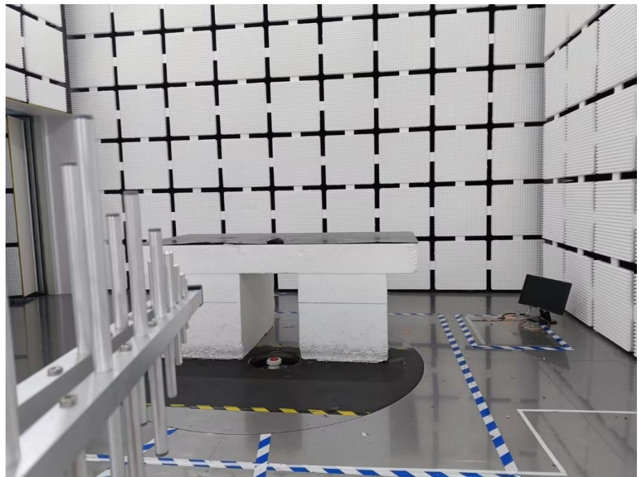
Radiation Emission Test Setup (30MHz to 1GHz)
