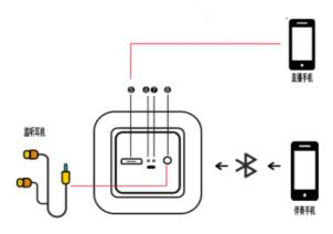
◆ Open the package and take out the microphone and accessories, connect one end of the audio cable to the 'DC5V' interface of KGObo, and connect the other end to the live
