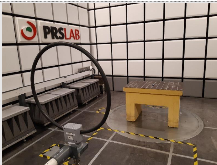
PHOTO N° 2 – SETUP FOR RADIATED MEASUREMENT
