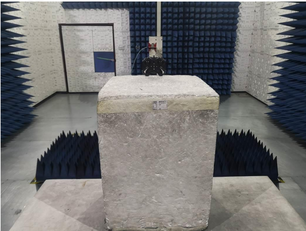
FCC RADIATED EMISSION TEST SETUP ABOVE 1GHZ
