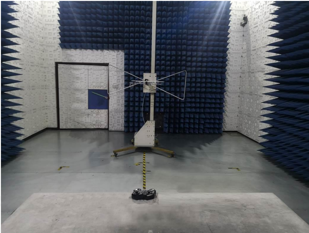
FCC RADIATED EMISSION TEST SETUP ABOVE 1GHZ
