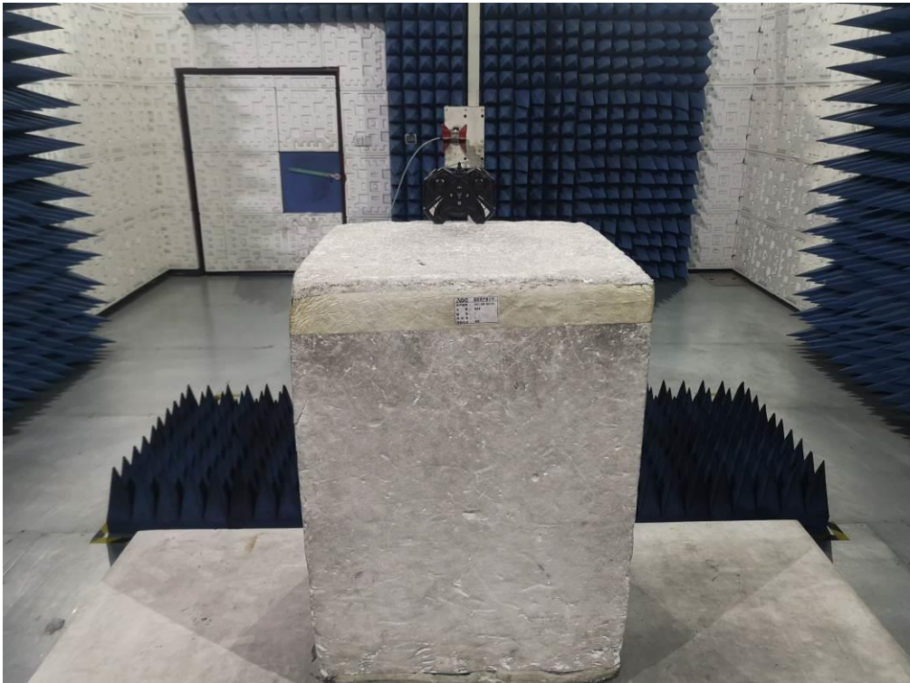
FCC RADIATED EMISSION TEST SETUP ABOVE 1GHZ
