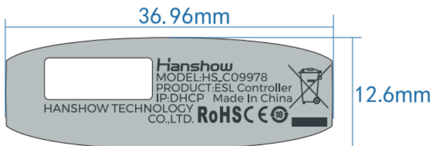
Figure 2-2 Nameplate of HS_C09978
