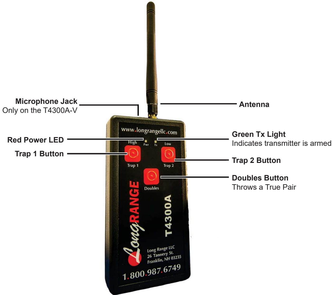
Press any button to power on the transmitter. Be aware that this first button press, even though the device is off, will fire the corresponding trap or traps. The **Red Power LED** will illuminate to let you know that the device is on and ready to launch the second target.
