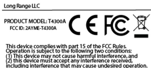
Specifications: The label shall be securely affixed to a permanently attached part of the device, in a location where it is visible or easily accessible to the user, and shall not be readily detachable. The label shall be sufficiently durable to remain fully legible and intact on the device in all normal conditions of use throughout the device's expected lifetime.
