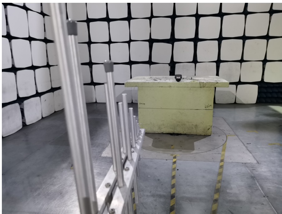
Radiation Emission Test Setup (30MHz to 1GHz)
