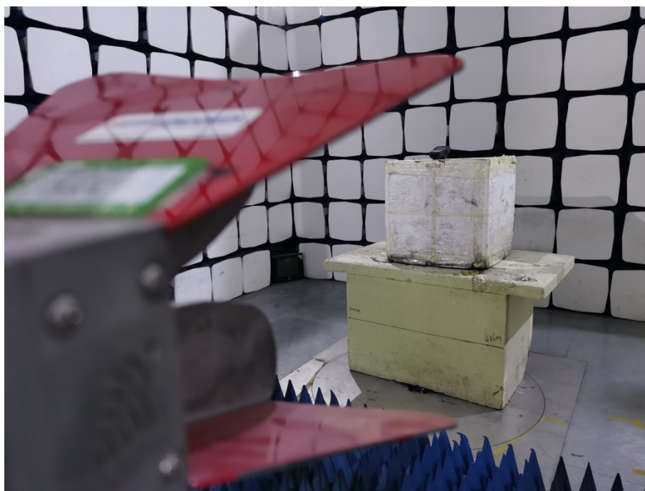
Radiation Emission Test Setup (1GHz to 18GHz)
