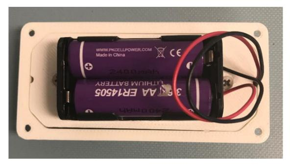
**Step #3:** Remove both batteries.
