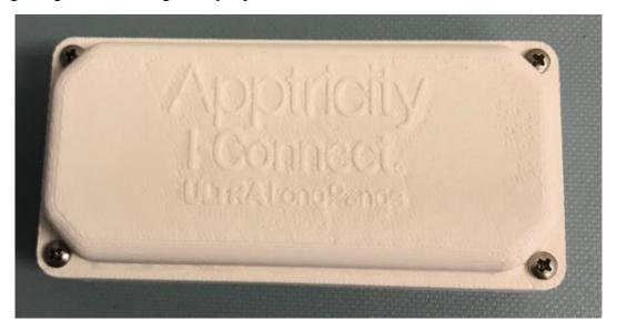
**Step #1:** Remove the 4 screws from the top of the case.
