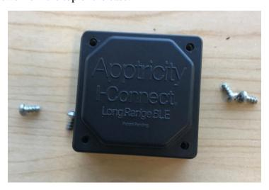
**Step #2:** Remove the lid with attached pcb from the case.
