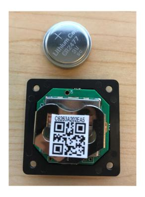
**Step #4**: Insert new battery with positive side up (very important) and negative side against the shield.
